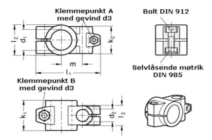
Adjustable clamp lever for d3 = GN 911-M 8-32 have to be ordred separately Adjustable clamp lever for d4 = GN 911-M 6-25 have to be ordred separately d1 = 30 d2 = 16 d3 = M 8 d4 = M 6 k1 = 40
